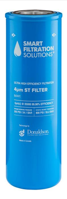
Smart Filtration Solutions Ultra High Efficiency Filters are designed with Donaldson's proprietary synthetic media to remove 99.98% of abrasive particulates in a single pass. All our filters are equipped with Viton® seals to have optimum compatibility with various fuels & oils.
