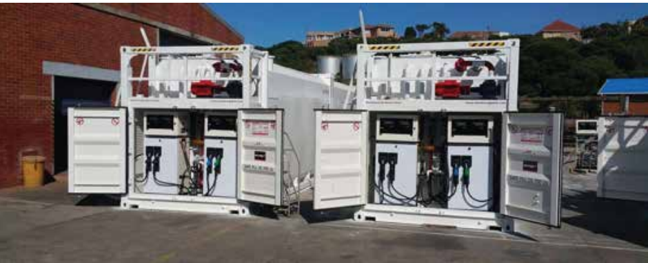
SPLIT COMPARTMENT TANKS. PETROL / DIESEL AND PARAFFIN
